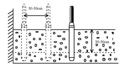
The concrete has been thoroughly vibrated when the surface around the poker vibrator becomes glossy and no large air bubbles break surface. This normally takes 10-20 seconds. Withdraw the vibrator slowly so that the concrete has time to flow back into the cavity left by the vibrator.
